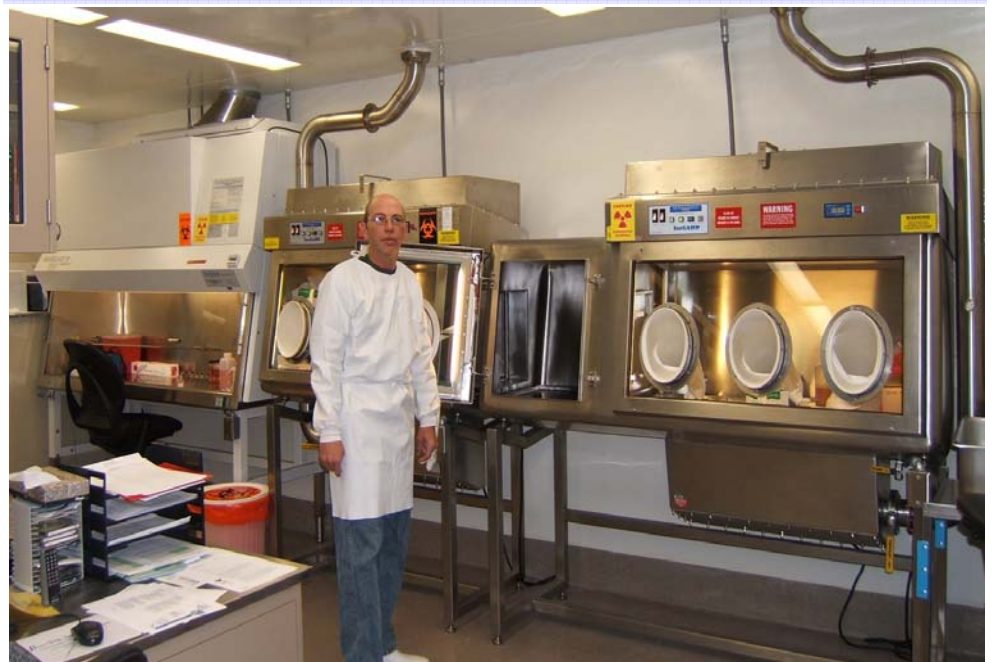
Joe Hattie of Michigan State University stands next to his Baker Class II and Class III Biological Safety Cabinets. Baker cabinets provide personnel, product, and environmental protection.
