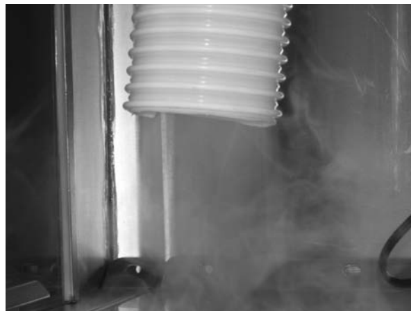
Figure 6: Microsphere aerosol for dynamic and cross-contamination test
