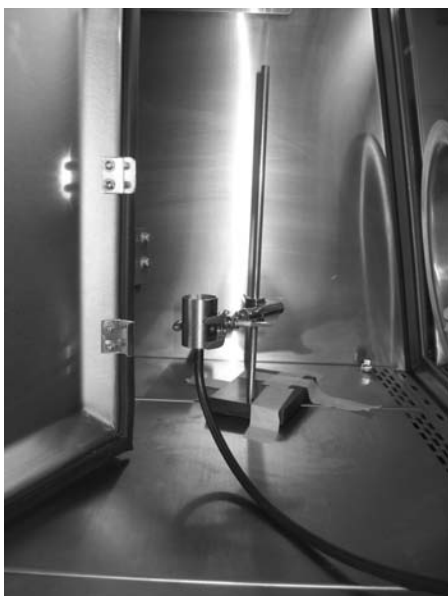
Figure 4: Particle counter sample probe (shown for ChemoSHIELD ingress/egress test)
