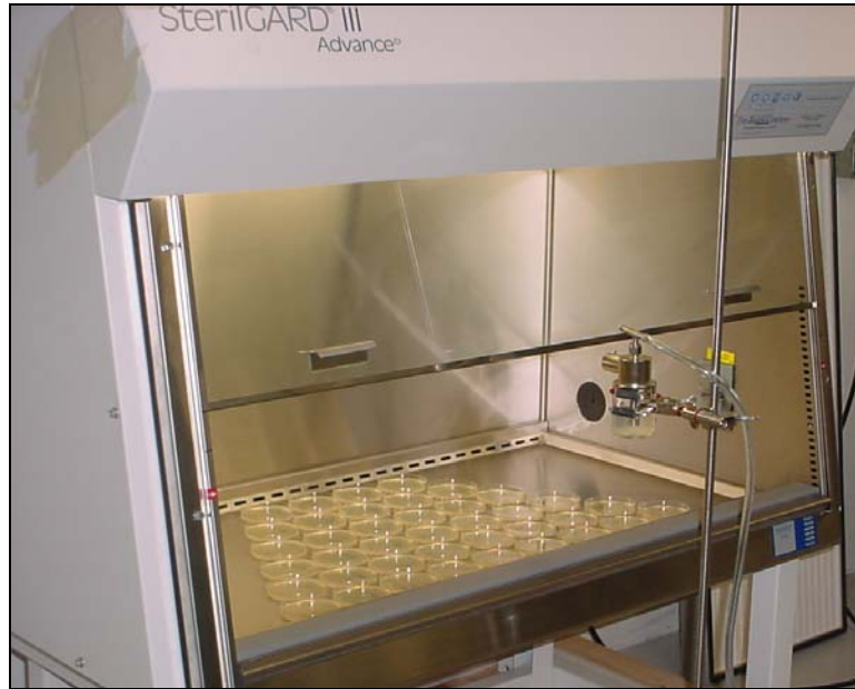
Figure 3. Product protection test for model SG403A HE with sash open at 12-inch height.
