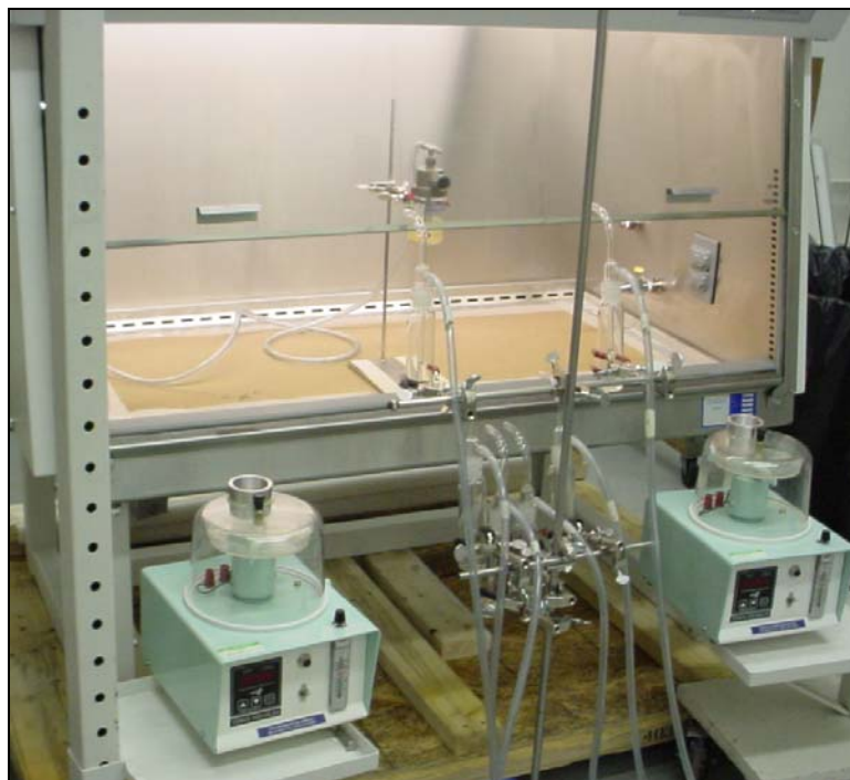
Figure 1. Personnel protection test for model SG403A HE with sash open at 12-inch height.
